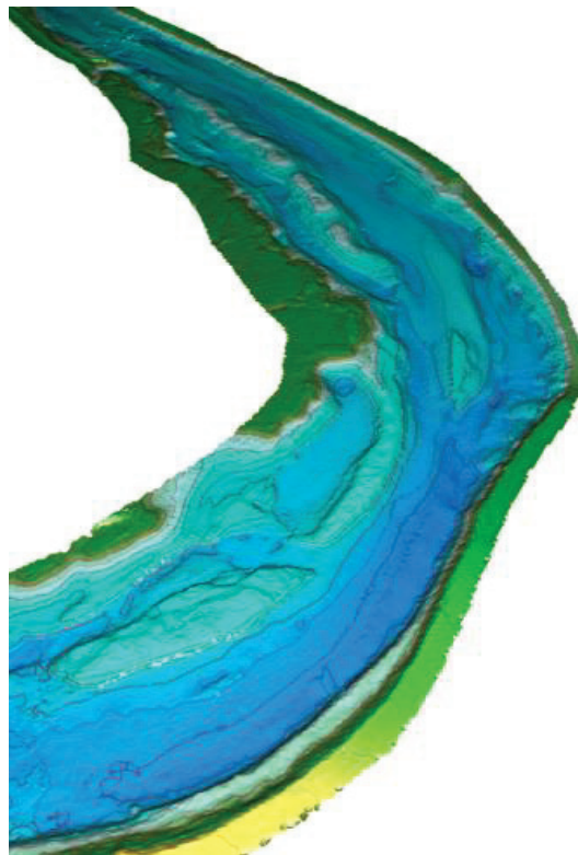
Figure 2: example of a bathymetric terrain model generated on basis of Hydromapping data (visualization with HydroVISH)
